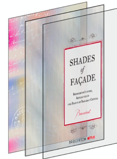
Multi-layer acrylic panel detail with printed graphics
